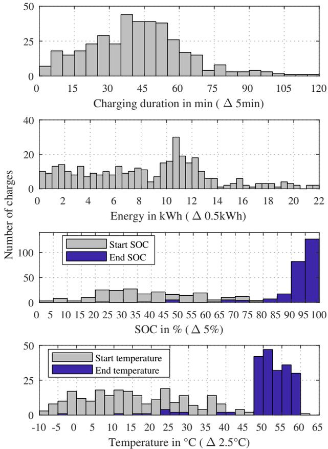
Fig. 6. Number of charges in the data set distributed by the charging duration, energy, start/end SOC and start/end battery temperature
