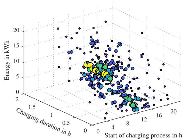
Fig. 4. Load behavior of the fast charging post
