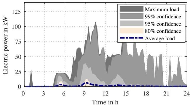
Fig. 7. Load profile of the Fraunhofer fast charging station
