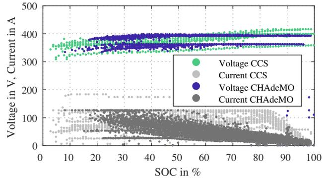
Fig. 12. Development of voltage and current over the course of charging
