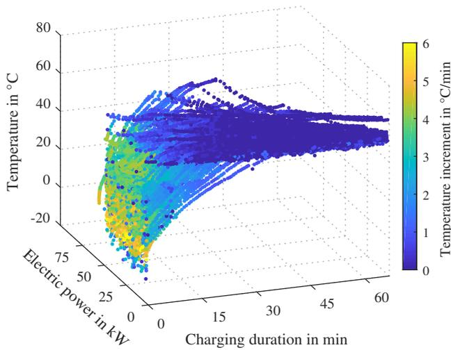
Fig. 11. Rise of battery temperature during a charge, differentiated by power
