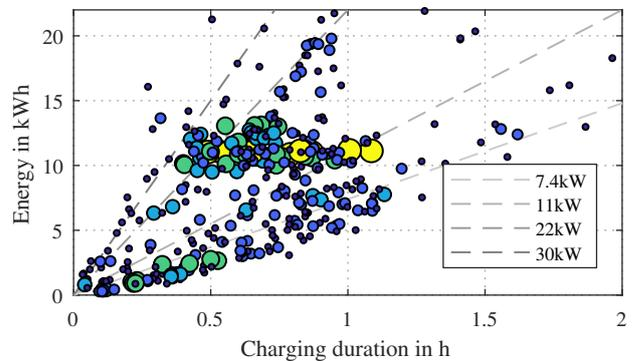
Fig. 5. Charging power of the fast charging post
