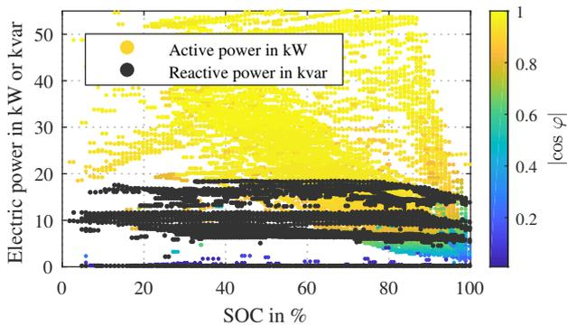
Fig. 13. Development of  $\cos \varphi$ , apparent and reactive power over the course of charging
