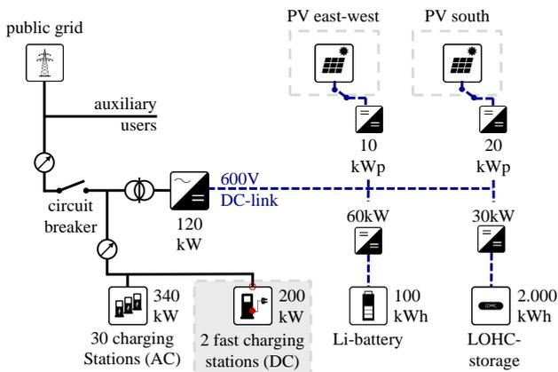
Fig. 2. Overview of the Fraunhofer Micro Smart Grid
